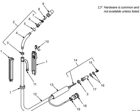
Figure 6-1. Complete Assembly (GA-16C Gun Illustrated)
